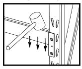
Be sure the load beam clips in step 1 remain locked.
