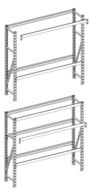
First install the back top load beam.
