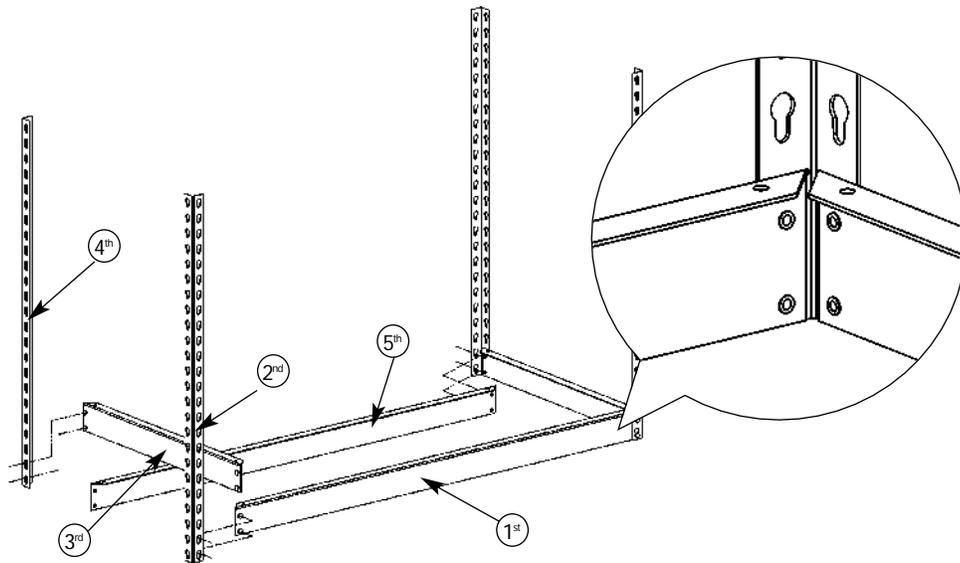
**Step 2 - Primary End and 36"Double Rivet Beams**
