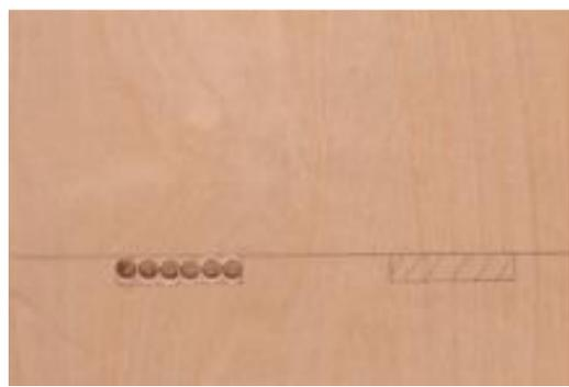
Grooves on the wood can very easily be cut out with a plate jointer, if you have one otherwise use a drill with 3/8" wood bit. Drill a few holes in the marked area 3/4" deep.
